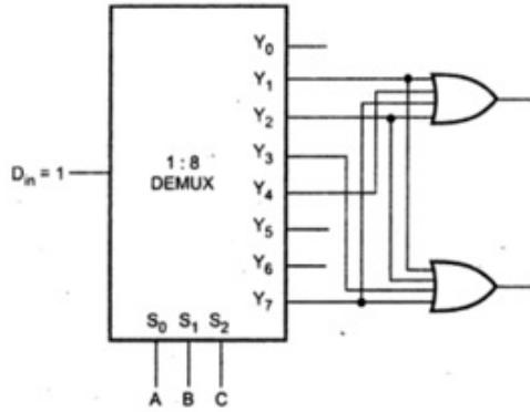
The circuit shown in the given figure represents a/an:
