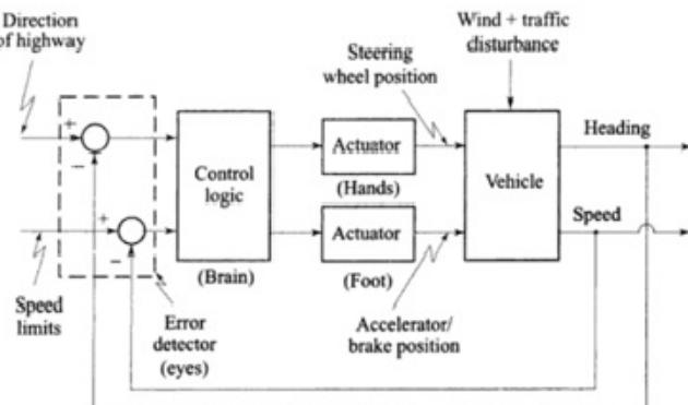
The control system illustrated in the figure is an example of a/an:
