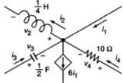
In the given figure,  $i_1 = -0.5e^{-2t}$ ;  $v_3 = 2e^{-2t}$  and  $v_4 = 5e^{-2t}$ . Find  $v_2$ .
