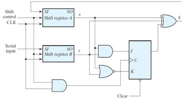
In the given figure, what will be the binary value in register A after two shifts for the serial adder which uses two four-bit registers? Register A holds the binary number 0101 and register B holds 0111.
