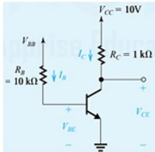
Find  $V_{BB}$  if the circuit (in the given figure) has to operate at the edge of saturation (Use  $V_{BE} = 0.7$  V and  $\beta = 50$ ).
