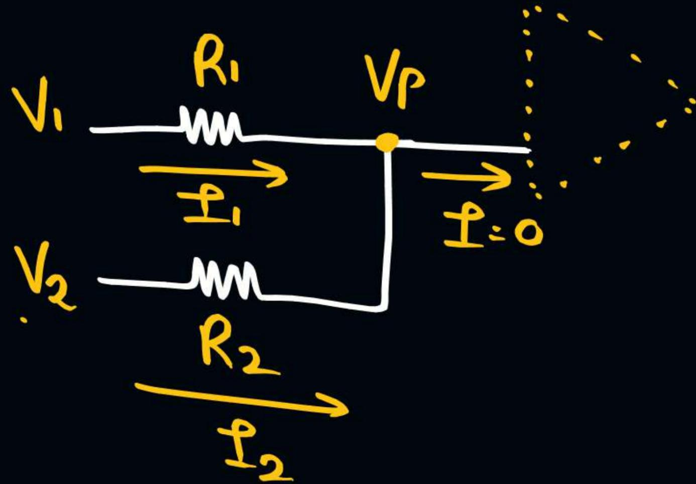
$$\frac{V_1 - V_P}{R_1} + \frac{V_2 - V_P}{R_2} = 0$$
