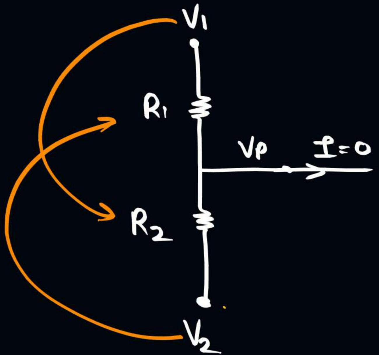
$$V_p = \frac{V_1 + V_2}{2}$$
