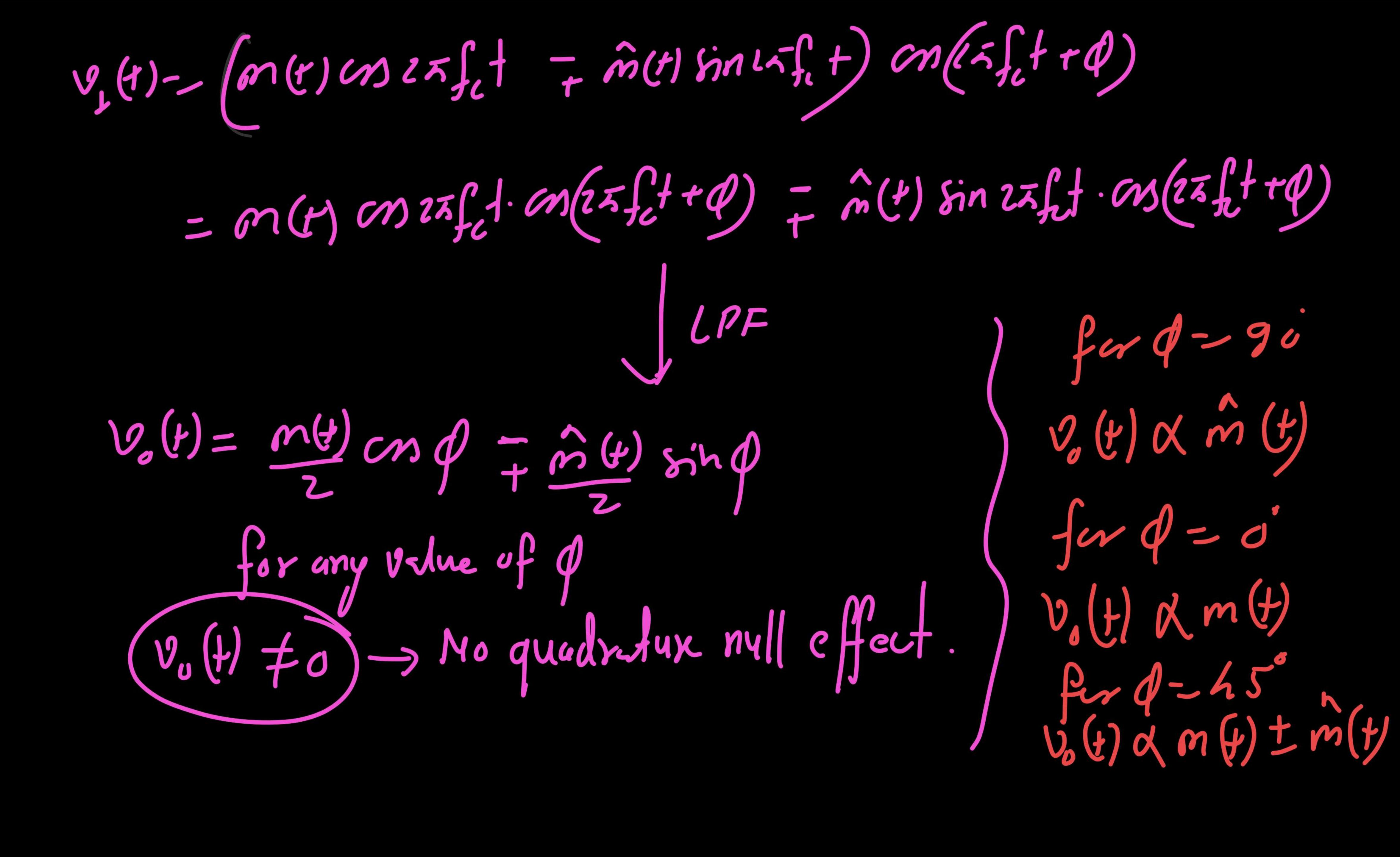
Adv: Bwisley Demodulation is always possible by Synchronous detector. No Quadrature Null Effect.
