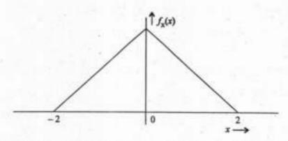
A low pass stationary process X(t) has probability density function (at any given point of time) as shown in the figure. This process has a bandwidth of 5 kHz and is to be transmitted by using a PCM system.
