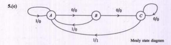
Construct the state diagram for a Moore circuit from the given Mealy circuit.
