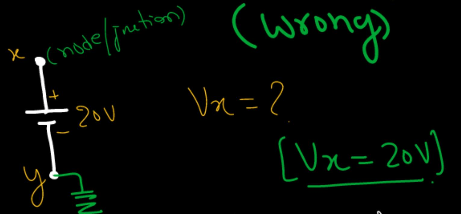
\* to calculate node Vol, one reference point is mandatory in the circuit.
