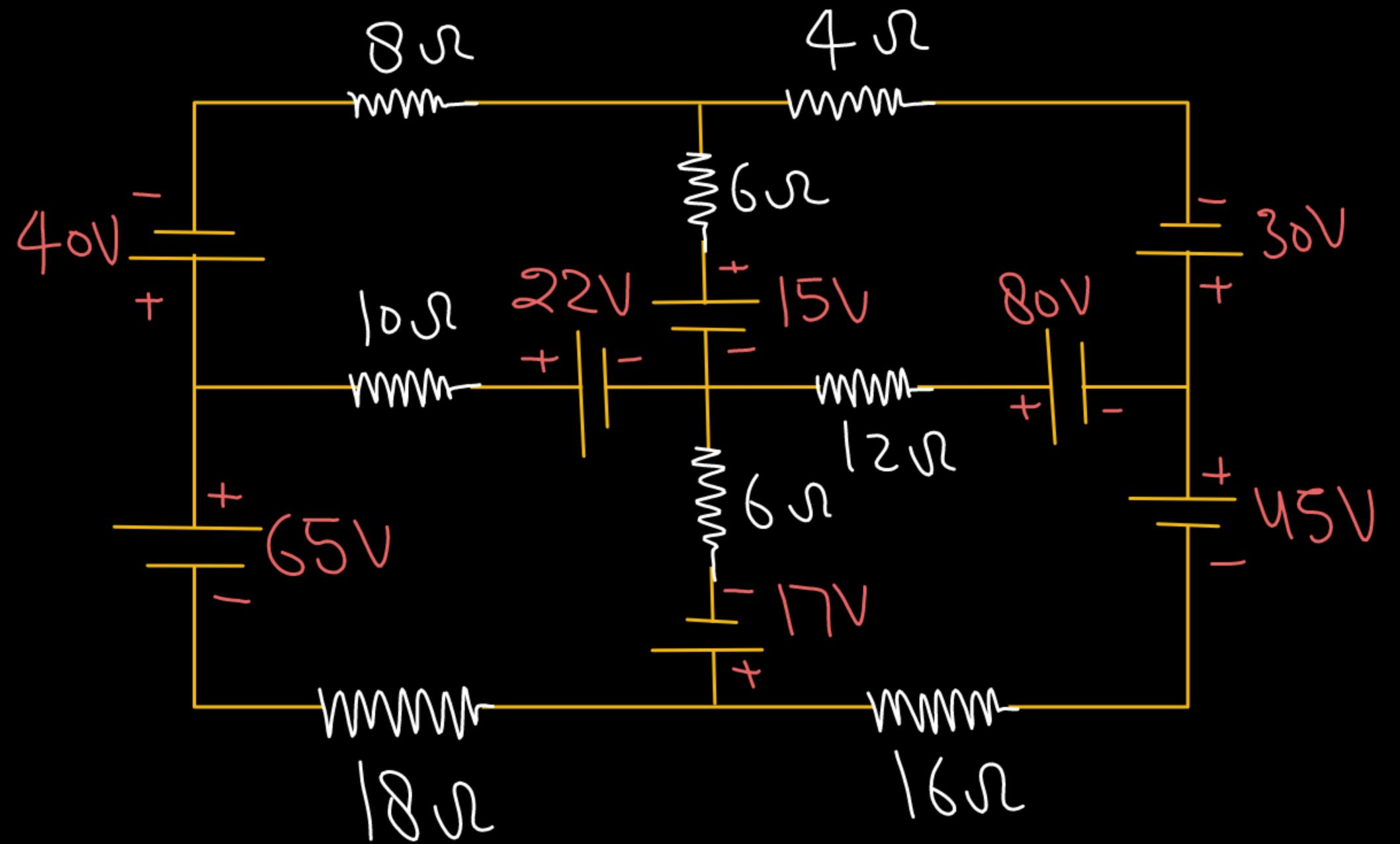
Ex. Write down all possible necessary KVL Equations .
