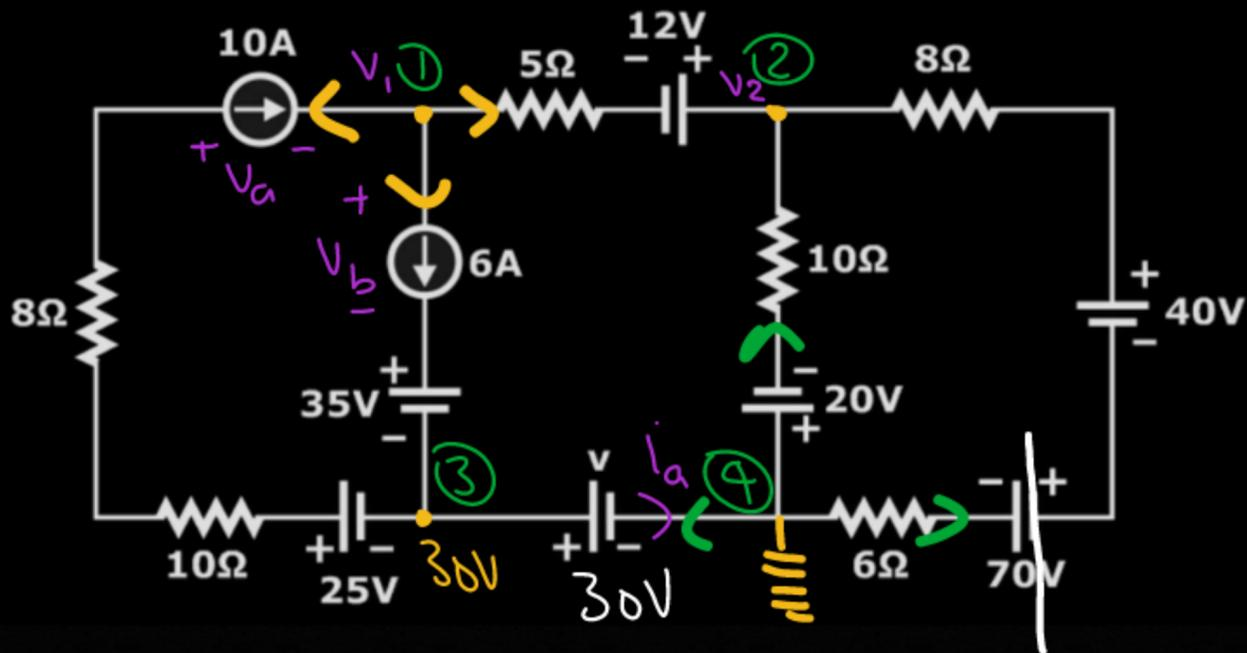
Ex. calculate power delivered by both current sources in given Circuit
