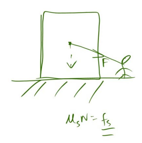
The block shown in the given figure is kept in equilibrium and prevented from sliding down by applying a force of 500 N. The coefficient of friction is  $\sqrt{\frac{3}{5}}$  The weight of the block would be
