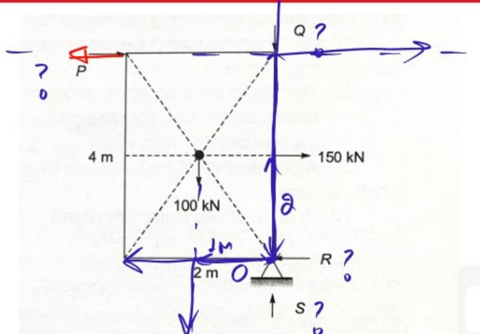
A rectangular plate is held in equilibrium by the application of forces as shown in the figure. What is the magnitude of the force *P*?
