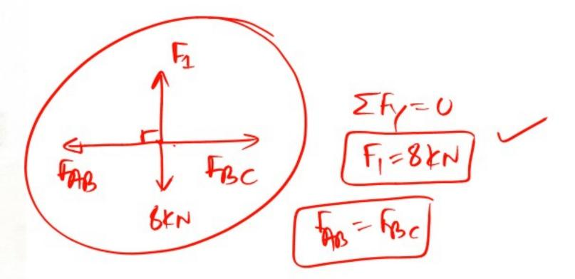
The given figure shows the loading pattern on a truss. The force in the member *AC* is
