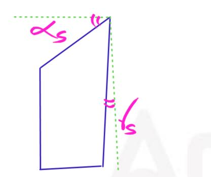
The angle of inclination of the rake face with respect to the tool base measured in a plane perpendicular to the base and parallel to the width of the tool is called
