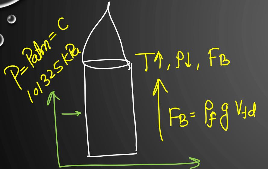
If the flow takes place naturally due to density difference i.e. due to Buoyancy Forces arising by change in density
