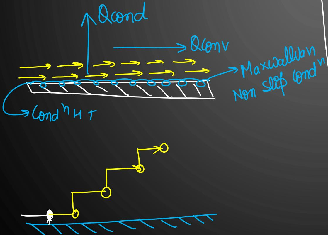
In Convection HT, HT by  $Cond^n$  is Transported by fluid (flowing)
