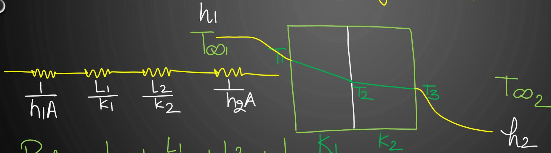
$$R_{th} = \frac{1}{h_1 A} + \frac{L_1}{k_1 A} + \frac{L_2}{k_2 A} + \frac{1}{h_2 A}$$
