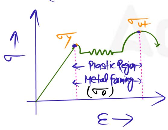
In the metal forming process, the stresses encountered are
