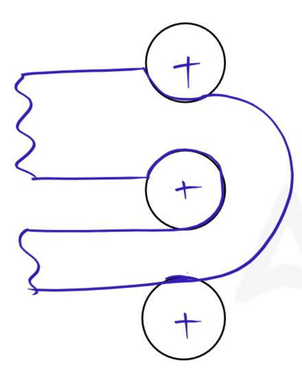
In one setting of rolls in a 3-high rolling mill, one gets
