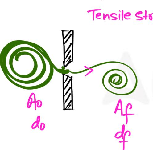
Which of the following types of stresses is/are involved in the wire-drawing operation?
