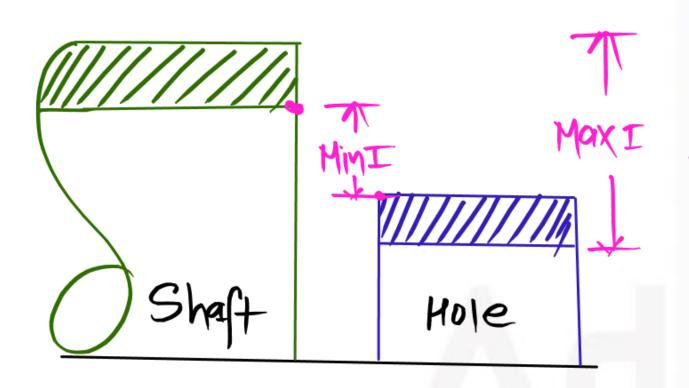
In order to have interference fit, it is essential that the lower limit of the shaft should be
