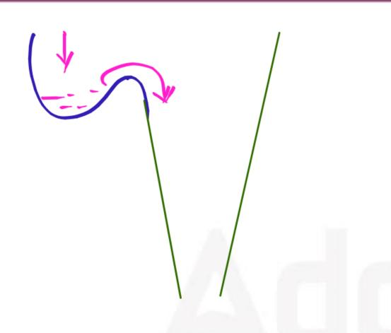
Converging passage is used for feeding the liquid molten metal into the mold to
