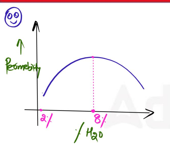
Increase in water content in moulding sand causes
