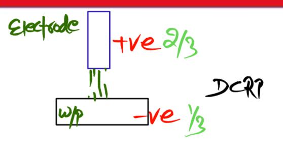
Submerged Arc welding Y under the flux
