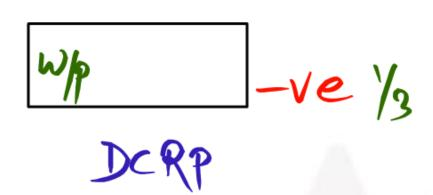
In arc welding d.c. reverse polarity is used to bear greater advantage in
