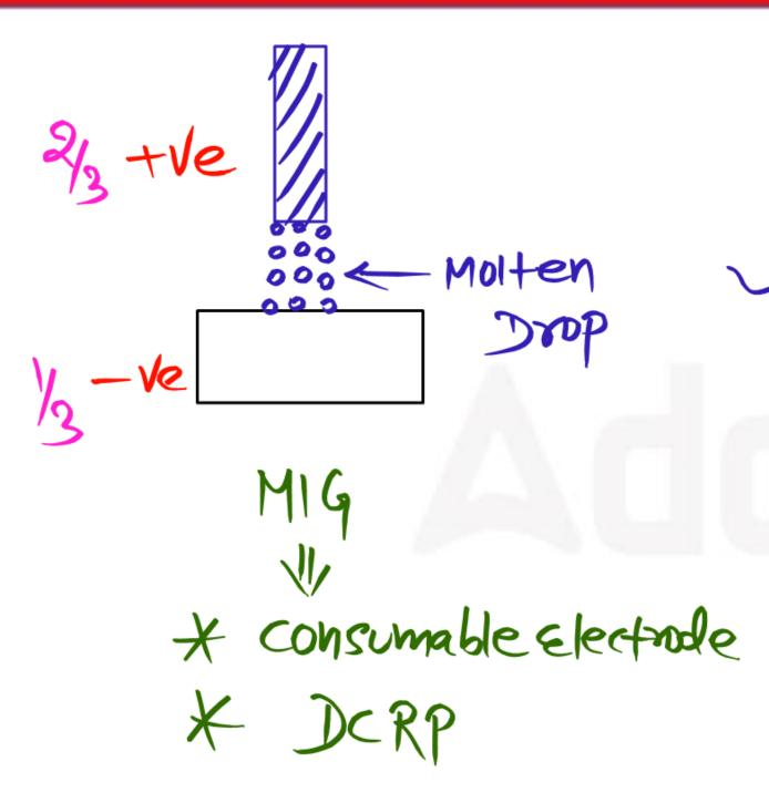
In MIG welding, the metal is transfered into the form of which one of the following?
