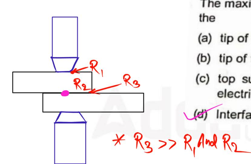
The maximum heat in resistance welding is at the
