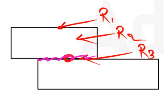
In resistance welding, heat is generated due to the resistance between
