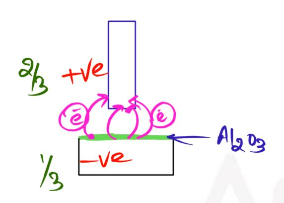
During plasma arc welding of aluminium, improved removal of the surface oxide from the base metal is obtained with typical polarity of
