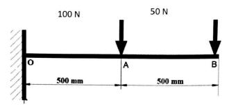
Given:  $E = 2 \times 10^5 \text{ N/mm}^2$ , Area moment of inertia of beam section = 10,000 mm<sup>4</sup>.
