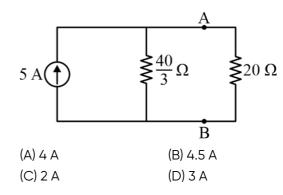
**Q93** Find the value of Load resistance  $(R_1)$  for maximum power transfer in the following circuit:
