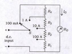
What are the values of resistances  $R_1$ ,  $R_2$ ,  $R_3$  and  $R_4$ , if the shunt resistances are connected as shown in the figure?
