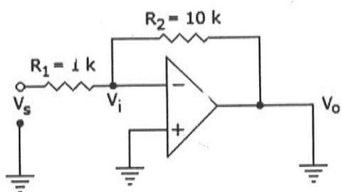
48. The  $V_o$  of the op-amp circuit of Fig. 5 is given as
