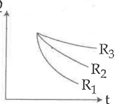
Three identical capacitors are given a charge  $\theta$  each and then they are allowed to discharge through resistance  $R_1$ ,  $R_2$  and  $R_3$ . Their charges, as a function of time shown in the graph. The smallest of the three resistance is :
