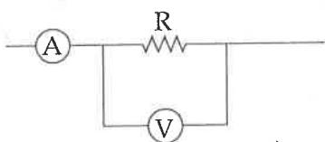
The ammeter A reads 2 A and the voltmeter V reads 20 V, the value of resistance R is :
