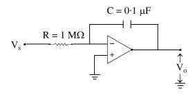
If  $V_s$  = 10 sin(1000  $\pi$ t) mV is supplied to the OPAMP circuit, given in the figure, then the value of the output  $V_o$  is
