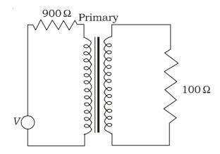
For maximum power transfer to the load, the primary to secondary turn-ratio may be
