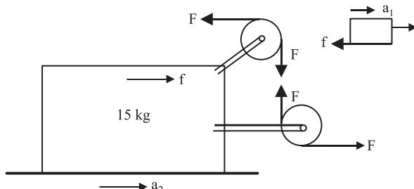
10 kg block will not slip over the 15 kg block till acceleration of 15 kg block becomes maximum as it is created only by friction force exerted by 10 kg block on it.
