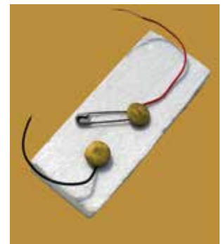
Figure 41.1 A simple switch
