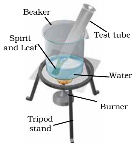
Figure 4.1 Set-up for extraction of chlorophyll
