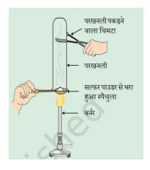
Pratyush took sulphur powder on a spatula and heated it. He collected the gas evolved by inverting a test tube over it, as shown in figure below.
