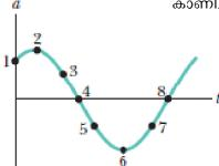
Which of the labeled points indicate, mean position, maximum velocity, maximum kinetic energy, and maximum acceleration **(4)**
