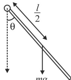
$T = 2\pi\sqrt{\frac{l}{g}}$  where  $l$  = length of simple pendulum = length of rod.
