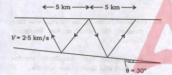
What will be the dip moveout for a single dipping reflector with 30° dip, beneath a homogeneous top layer of velocity 2.5 km/s?
