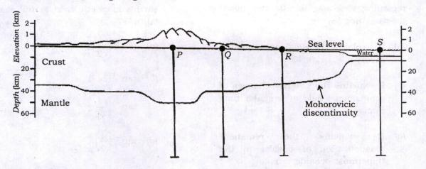
Assuming that the measured gravity is equal to the normal gravity value, which point in the above diagram has zero Bouguer gravity value?
