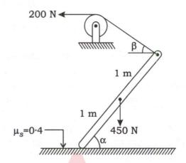
A rod of length 2 m and weight 450 N rests on ground at one end. The other end is supported by a cord through which a force of 200 N is applied. What is the minimum angle  $\alpha$  for which equilibrium is possible? The coefficient of static friction between the rod and the floor is 0.4:
