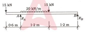
Determine the deflection at a point 1 m from the left-hand end of the beam loaded as shown in the figure below. Use double integration method. The beam is having a constant flexural rigidity of 0.6 MN-m<sup>2</sup>:
